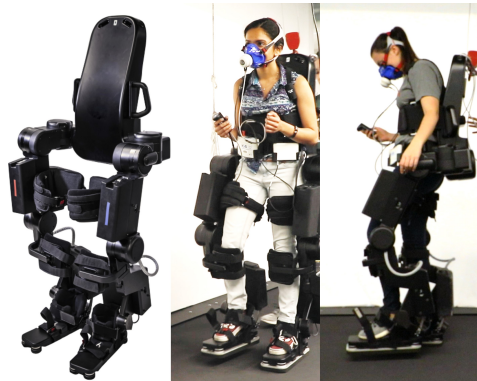
Fig. 1. Atalante Exoskeleton with and without the user. The user is wearing a mask to measure metabolic expenditure.
